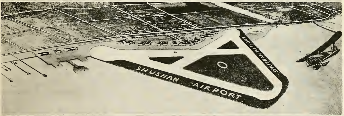
Plan of the 310-acre landplane and seaplane airport being built into Lake Pontchartrain at an initial expenditure of $2,000,000
